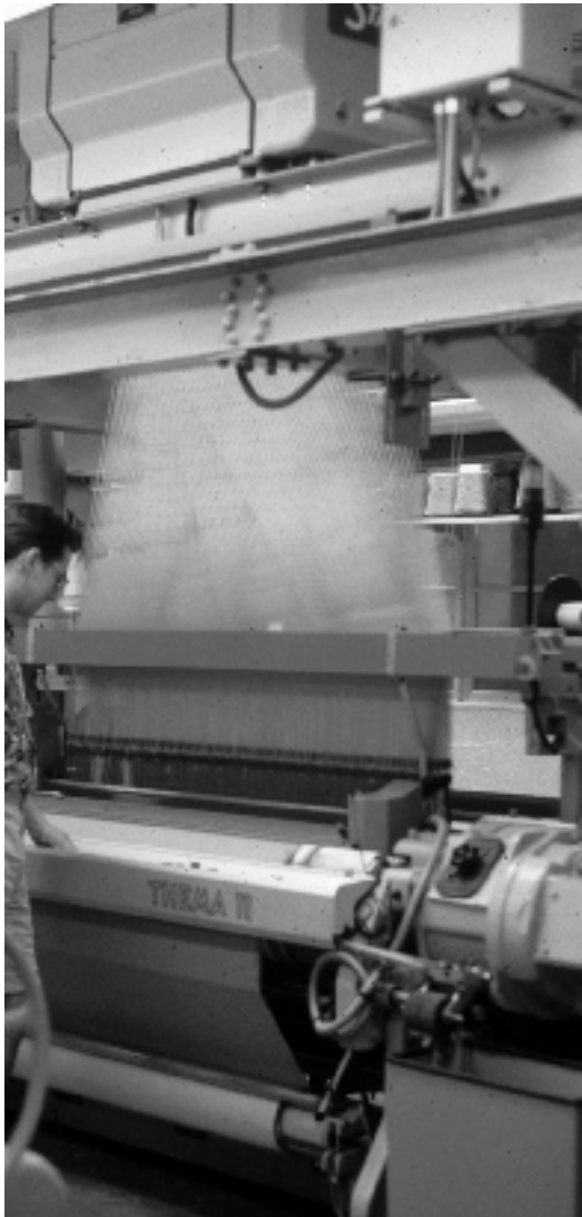
I-9 Stäubli Jacquard Controller on a Somet Electronic Loom
